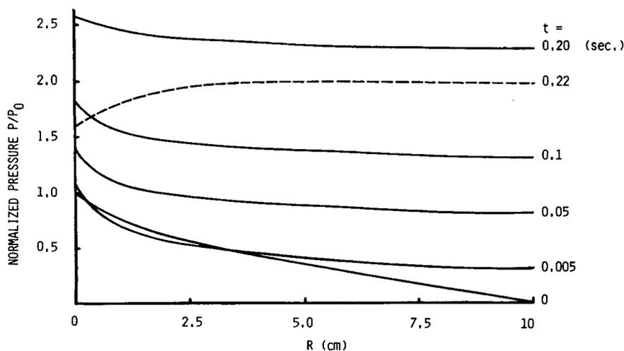
Fig. 1. Pressure buildup in the disk cavity for polystyrene.
