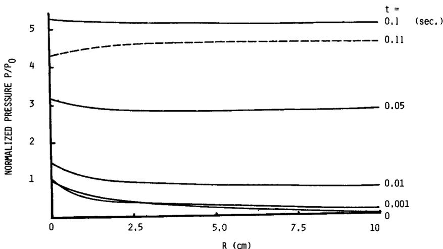
Fig. 2. Pressure buildup in the disk cavity for polyethylene.
